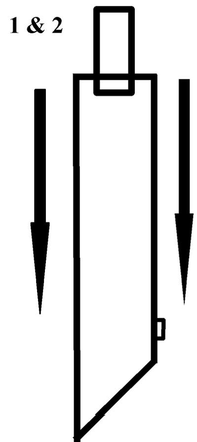
1. Remove screw and spry WD 40 in both the inlet and exit end of the muffler. This is to help release the baffle from the muffler housing and will not damage the baffle or the muffler housing so use a lot and go around the outside of the baffle.
