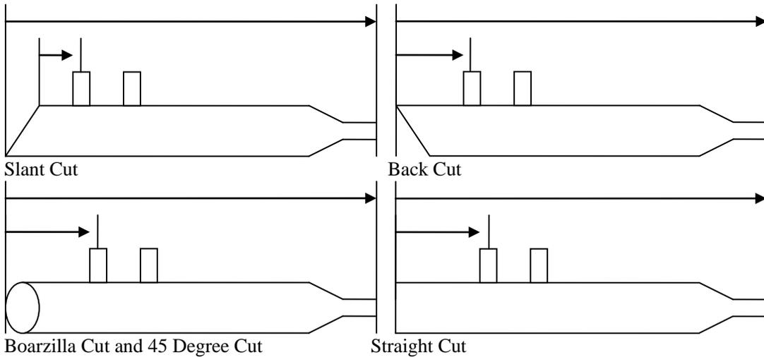
**Measure from the center of muffler stud to the end of the muffler depending on the cut you want. You don't have the measure the length of the whole muffler just from the center of back stud to the end of the muffler.**
