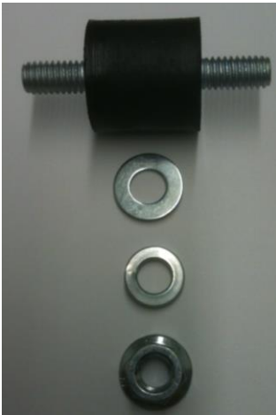
Hardware to mount to stock starter bracket
