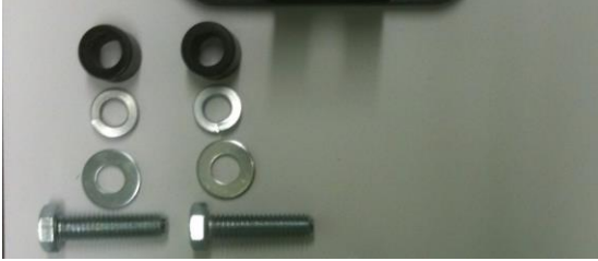
Muffler Bolts and Spacers
