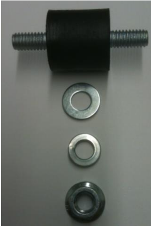
Hardware to mount to stock starter bracket
