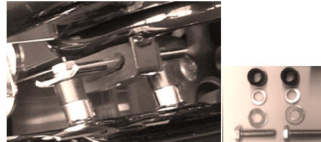
Muffler Bolts and Spacers W 1/2 OD Round 5/8 ID 3/8 5/16-18 x 1 1/4 Hex Bolt, Flat Washer, Lock Washer
